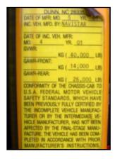
Figure 93. Secondary Manufacturer GVWR Plate
