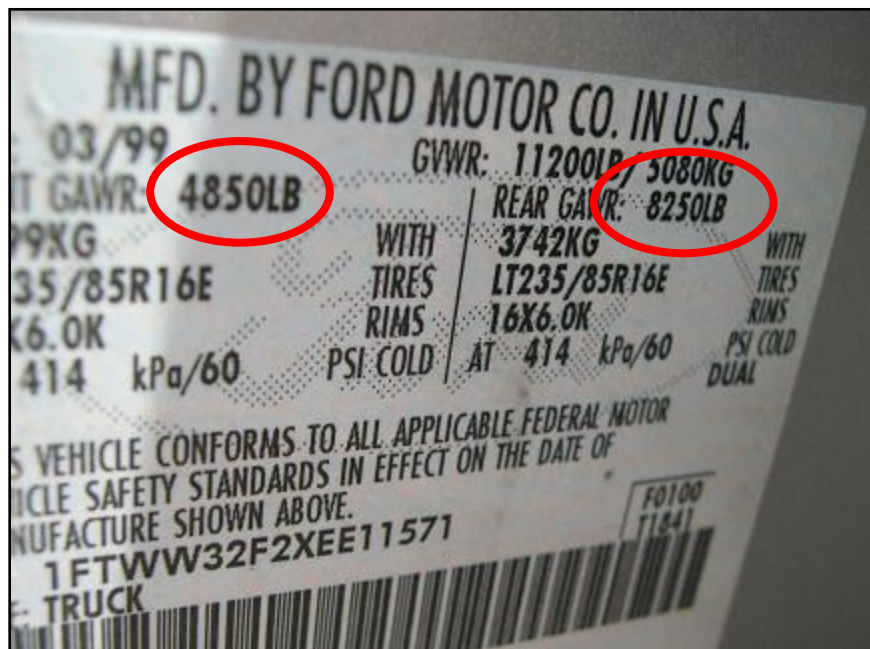
Figure 92. Front and Rear Gross Axle Weight Rating
